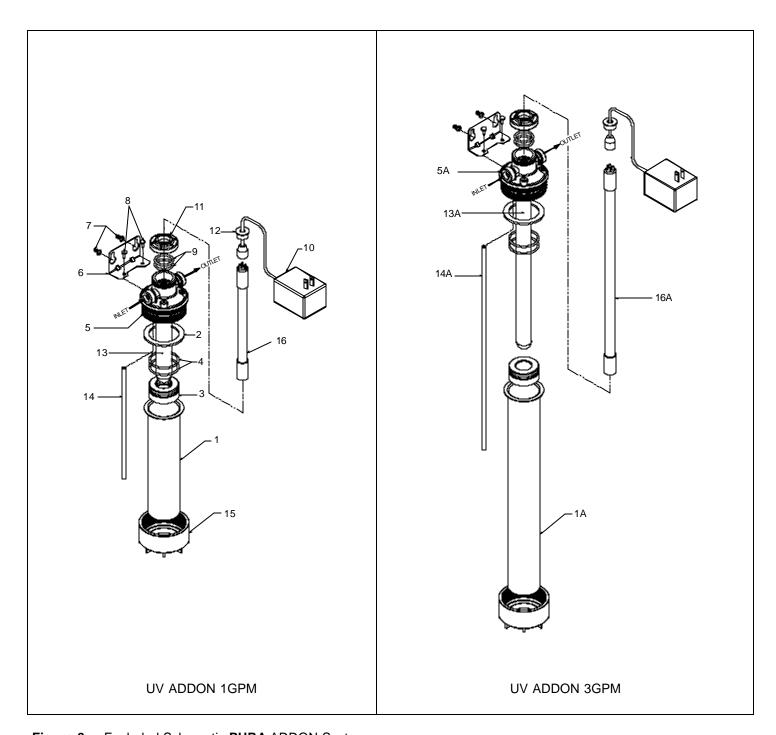
Figure 8 Exploded Schematic PURA ADDON System
