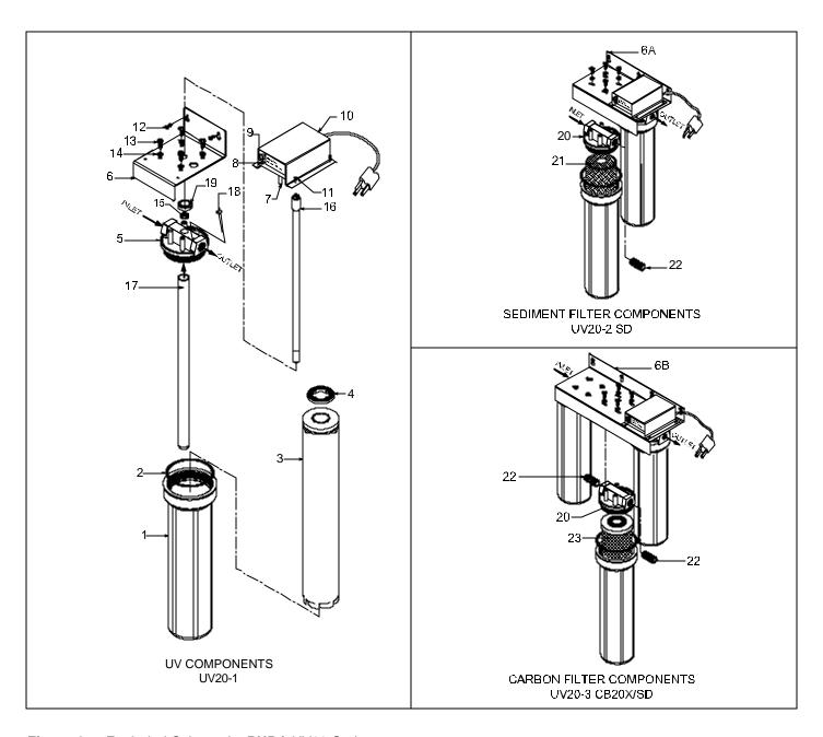
Figure 2 Exploded Schematic, PURA UV20 Series
