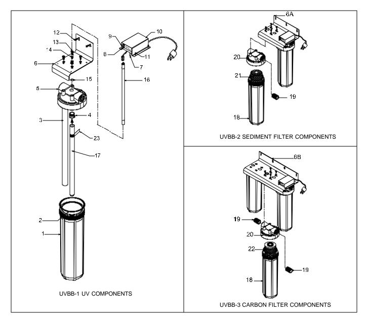
Figure 3 Exploded Schematic, PURA UVBB Series
