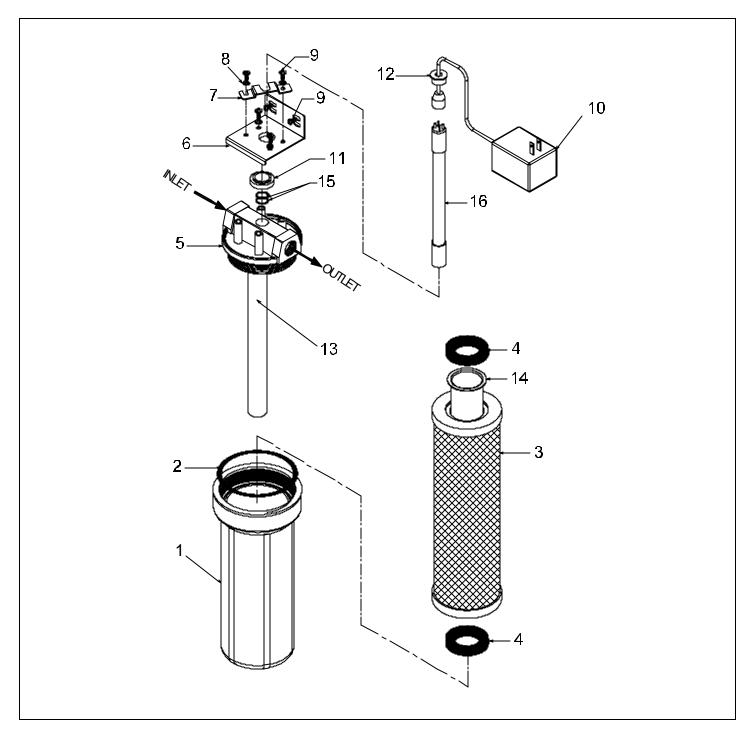
Figure 7 Exploded Schematic, PURA UV1Series
