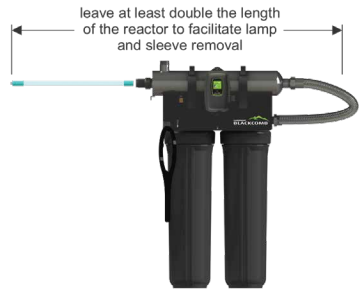
Figure 3. Lamp Removal Spacing
