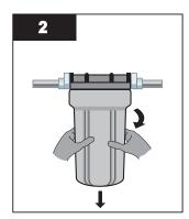
Unscrew sump from outer head and remove cartridge emptying water from sump.
