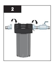
Screw filter to the adapter after covering the threads with Teflon® tape and make a tight connection but do not over tighten.
